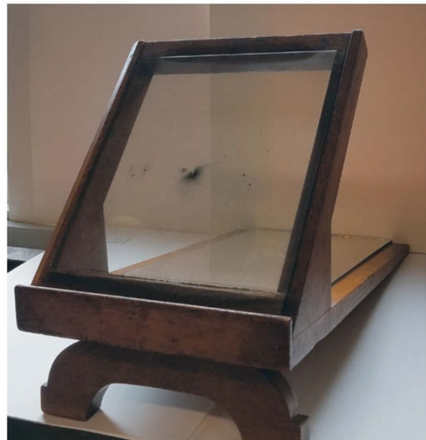
▲ VIEW FINDER Specially constructed light lecterns held the glass plates in place for close study. Illumination came from below, via a mirror that caught daylight from a window and directed it up through the glass image to the observer's eye.
